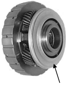
Oil Slinger on a Gear Figure 6
