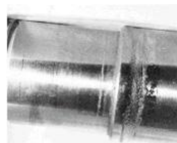
Overloaded bearing wear damage to shaft Figure 14 C
