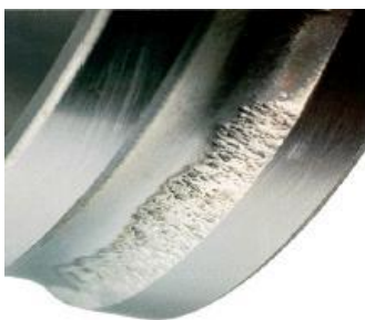
Overloaded bearing in axial direction Figure 14 A
