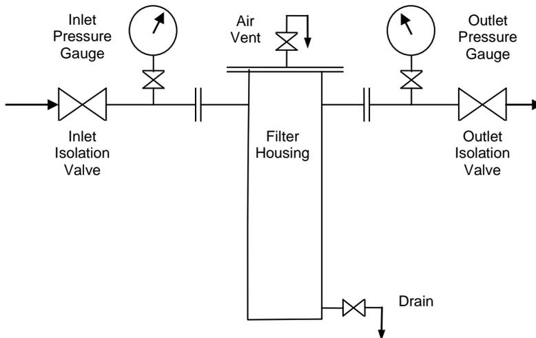
Figure 6 Minimum Filter Station and Strainer Design
