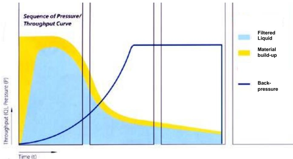
Figure 4 Effects of Material Build-up on Back Pressure and Liquid Flow Through a Filter
