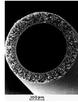
Figure 5 Filter Membrane Element Section Cross-Sections
