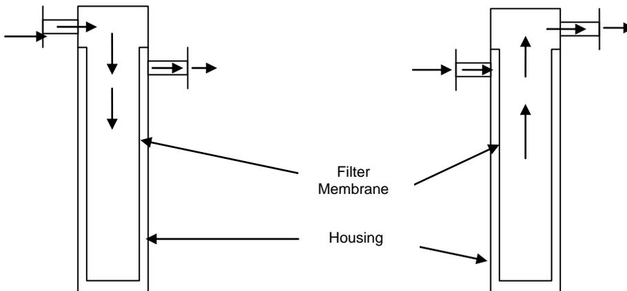
Figure 7 Liquid Flow Down Through Screen
